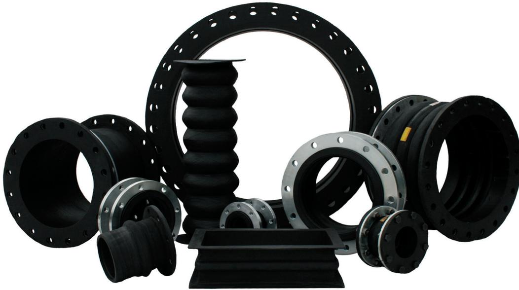
Unaflex rubber expansion joints provide relief from stresses caused by thermal expansion and contraction in pipelines. Movement is always experienced in piping systems due to varying ambient temperatures, differences in temperature of materials handled, and differences in composition. Expansion joints absorb this movement and mitigate the risk of buckling or pulling apart.
